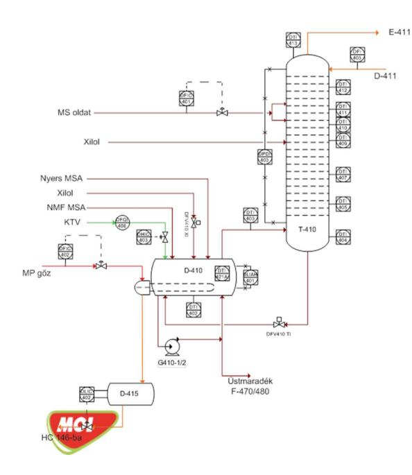
The distillation is not continuous but batch process and consists of several steps:
