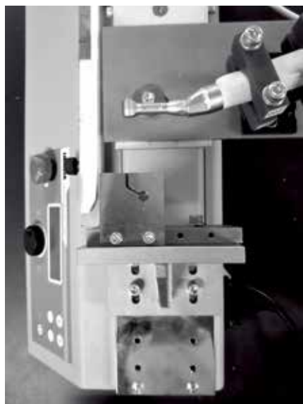
Fig. 1 Custom-made dynamic cyclic fatigue testing device used in the present study
