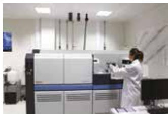
Left - Fig. 4: The Thermo Scientific HR MC ICP-MS at the STAIG lab Right - Fig. 5: A view into one of the ultra-clean STAIG prep. labs
