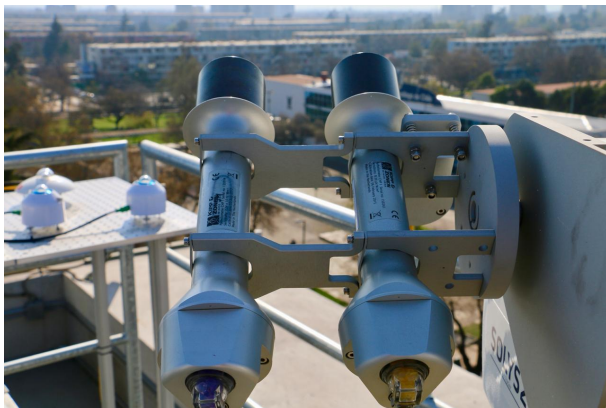
Figure 6. LES Pyrhelimeters deployment at USACH platform. Santiago Chile, September 5, 2018.
