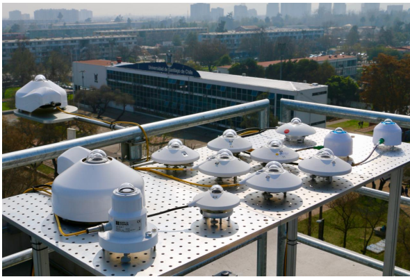
Figure 2. Pyranometers deployment at USACH platform. Santiago Chile, September 5, 2018.
