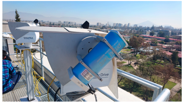
Figure 7. USACH’s PMO6-cc absolute cavity pyrhelimeter deployment at USACH platform. Santiago Chile, September 5, 2018.
