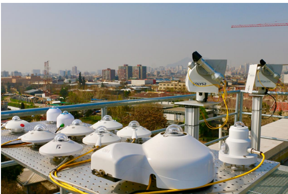
Figure 1. Pyranometers and pyrhelimeters deployment at USACH platform. Santiago Chile, September 5, 2018.
