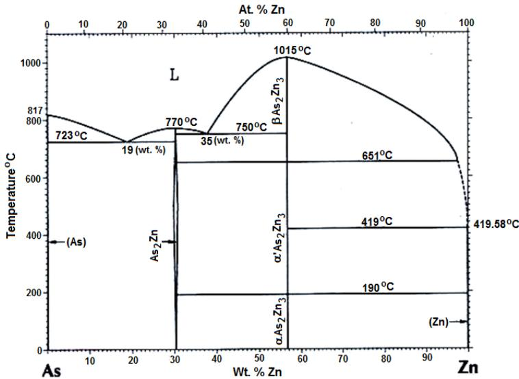
Figure 3. The Zn-As phase diagram (Okamoto, 1992) [15].
