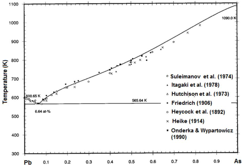
Figure 14. Optimized As-Pb phase diagram with experimental points [44].
