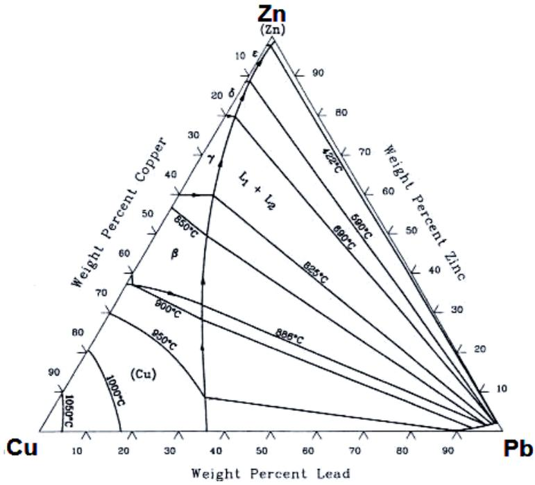
Figure 30. Cu-Zn-Pb liquidus projection (Okamoto, 1992) [79].
