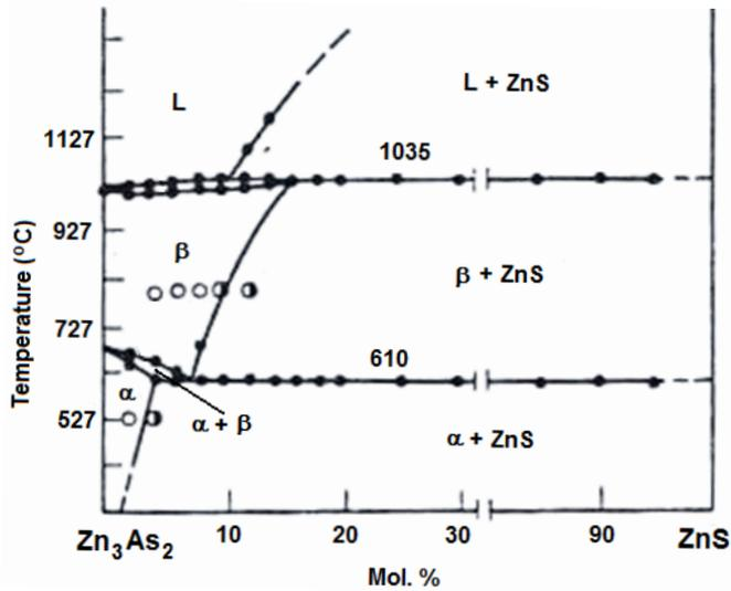
Figure 5. Phase diagram of the pseudo-binary  $\text{Zn}_3\text{As}_2$ -ZnS system [19].
