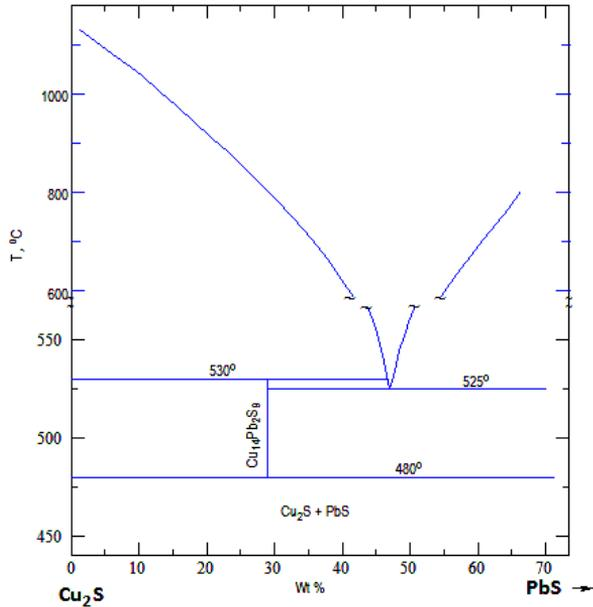
Figure 23. Phase diagram of the system Cu<sub>2-x</sub>S-PbS [41] (data from [82]).
