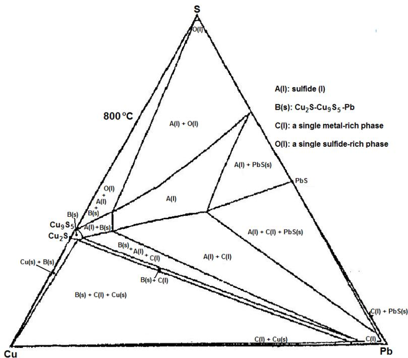
Figure 27. Phase relation in the system Cu-Pb-S at 800 °C, modified from Cho & Won [87].
