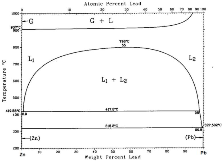
Figure 18. Phase diagram of the system Zn-Pb [57].
