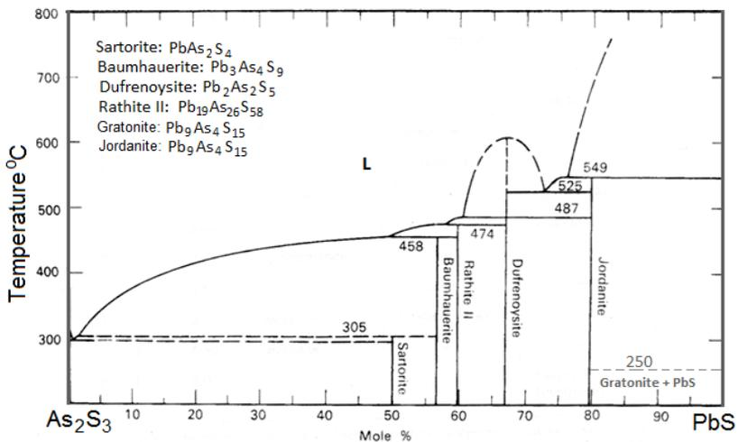
Figure 16. Phase relations in the binary  $As_2S_3$ - $PbS$  system (modified from Kutoglu (1969) [54] with gratonite/Jordanite transformation temperature, taken from Roland (1968) [51]), compositions are rough estimates based on both compositions in the diagram and reported minerals and compounds.
