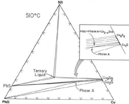
Figure 21. Phase relations in the condensed Cu-Pb-S system at 510 °C. Relations surrounding phase A ( $\text{Cu}_{14}\text{Pb}_2\text{S}_{9-x}$  ( $0 < x < 0.15$ )) are magnified, schematically in the insert [61].
