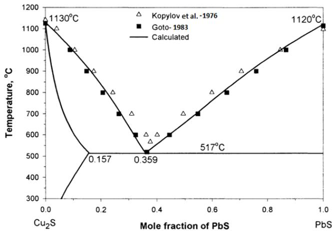
Figure 24. Calculated pseudobinary phase diagram of the system Cu<sub>2</sub>S-PbS with experimental points [84].
