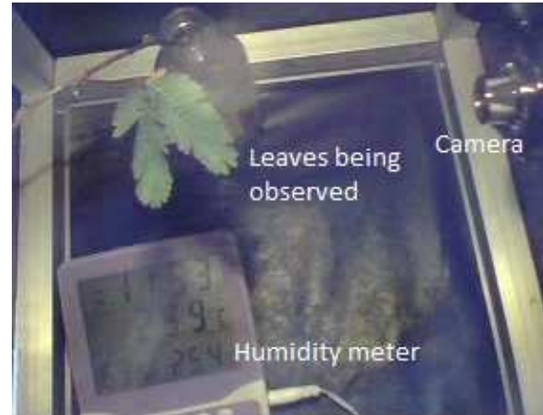
Fig. 3. Measurement set up of Puteri Malu in the box.
