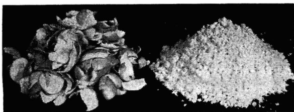
Figure 3. Navel Orange Peel before and after a 1-Minute Treatment on Mincing Apparatus
