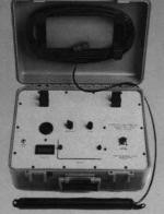
MG-230 Magnetic Gradiometer
