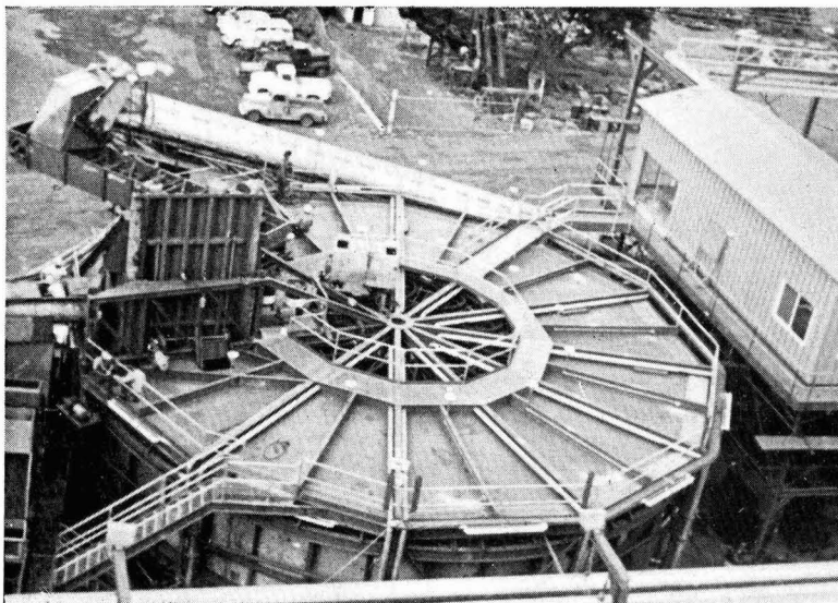
Fig. 5. Top view of the diffuser showing the prepared cane feed point and housing for the bagasse discharge.
