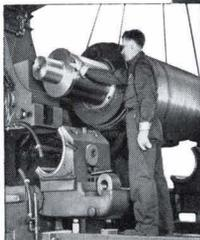
Patented side-cap construction permits fast vertical roll removal.
