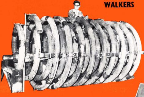
BATCH CRYSTALLIZER COIL ELEMENTS IN COURSE OF ASSEMBLY.
