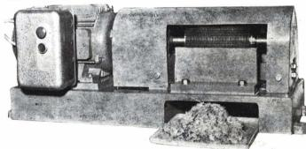
Our hot water digester for determination of the sucrose lost in bagasse, electrically heated, for 500 grm. samples. Other types for 500 and 1000 grm. samples include for direct heating or steam heating.
