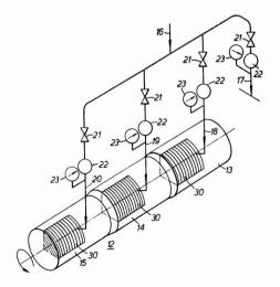
Water is admitted from pipe 16 through valves 21 to pipes 17, 18, 19, 20 delivering to the feed hopper and the three sections, respectively, the flow and pressure being indicated by meters 22, 23. The water is added by means of suitably drilled bars 30 which allow its passage under pressure into the bagasse or cane within the cage. The illustration shows water added at all three stages; they can be supplied individually with the recirculated press juices.
