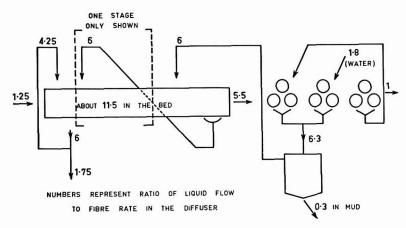
Fig. 5. Liquid balance in Fairymead diffuser
