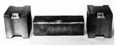
Fig. 7. Square shaft and coupling box
