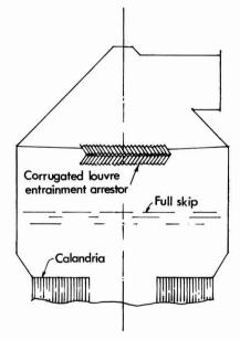
Fig. 3. Typical arrangement of corrugated louvre entrainment arrestor in a vacuum pan.
