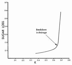
Fig. 2. Performance of corrugated louvre entrainment arrestor (based on trials on C.S.R. Co. Ltd. evaporator installations.) Sugar loss is expressed in lb/hr/sq.ft, arrestor area, where arrestor area is the horizontal projection of the opening through the arrestor. Coefficient K = lb vapour/sec/sq.ft, arrestor area  $\div \sqrt{(density \text{ of liquid})} \times (density \text{ of vapour}) (lb/cu.ft.).$
