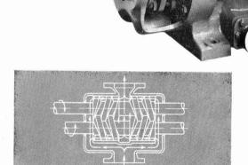
The two screws that provide the drive for Houttuin positive rotary displacement pumps, intermesh smoothly without metal to metal contact.
