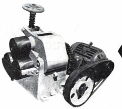
Our **ROLEX** laboratory three-roller mill is provided with 5 in.  $\times$  5 in. rollers of Meehanite cast fron, while the spur gears and casting which carries the adjustable top roller are of steel. This top roller is fitted with a compression spring while scrapers are provided for both bottom rollers. Oilite bearings are fitted, and the juice tray and scrapers are removable for cleaning. The illustration shows a **ROLEX** mill belt-driven by a 3 h.p. electric motor.
