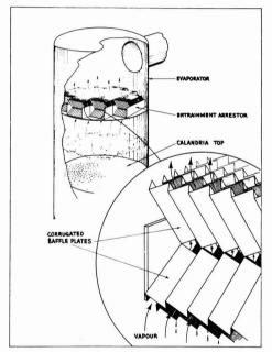
Fig. 1. Typical arrangements of corrugated louvre entrainment arrestor in final evaporator vessel. (Patent application for this invention has been filed in various countries.)
