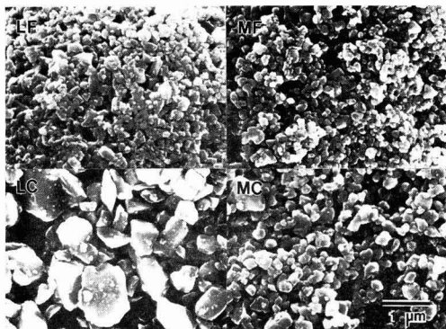
Fig. 2. SEM photographs of classified powders.
