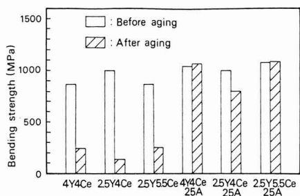
Fig. 12. Bending strength of (Y, Ce)-TZP and (Y, Ce)-TZP/Al 2 O 3 composites sintered at 1500°C before and after hydrothermal aging at 180°C and 1MPa for 35h.
