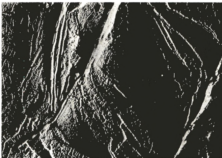
Fig. 8. Replica from free surface after xylene-stream exposure. Partial dissolution of the polyethylene surface lamellae is observed ( \times 21,000 ).
