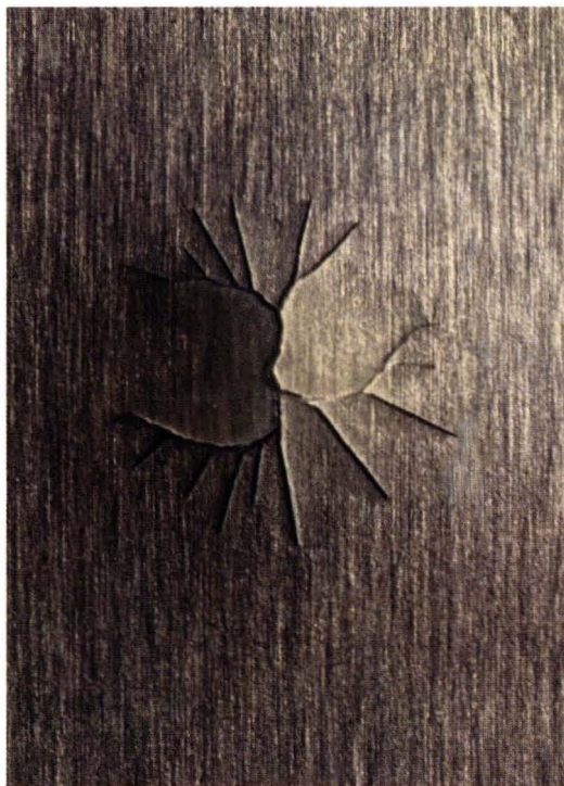
Coating without Hycar® RLP shows significant damage.
