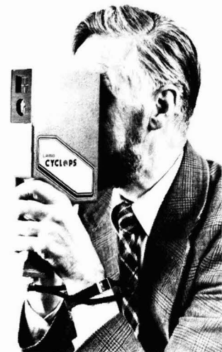
The Cyclops portable infrared thermometer from Land Pyrometers Ltd
