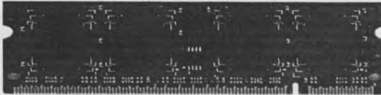
Fig. 11.14. 1GB DDR2 module in 204-pin SO-DIMM package
