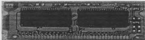
Fig. 12.12. SDRAM module in a 72-pin SO-DIMM package
