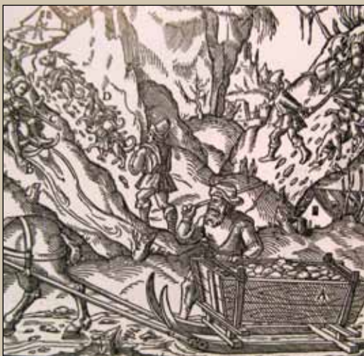
Slika 27: Transport rude nekoč: vleka sani s konjem, samotežne sani, psi nosači, v bisagah na ramah (Georg Agricola, De re metallica , 1556).
