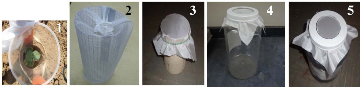
Figure 1. Five types of thrips cages evaluated: 1) transparent plastic cup cage, 2) wire mesh sleeve cage, 3) opaque plastic cylinder, 4) transparent plastic jar without ventilation, and 5) transparent plastic jar with ventilation.
