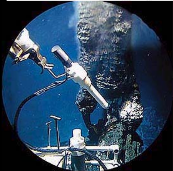
This wand extended from the deep-sea sub Alvin houses a thermometer, electrodes for taking chemical measurements, and an apparatus called the Sipper for collecting small water samples at hydrothermal vents.
