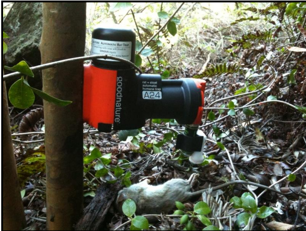
Figure 8. Goodnature® A24 Automatic rat trap with CO 2 cartridge and digital counter. Photo taken at Pahole NAR.
