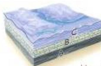
Subsidence below the sea and sedimentation of E over C; erosion surface of C preserved as an unconformity
