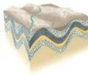
Subsidence below sea level and younger sediments deposited on former erosion surfaces
