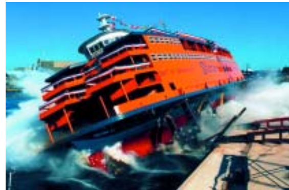
Marinette Marine recently installed new launchways that will enable it to build larger and more sophisticated vessels such as this 310-foot coastal ferry.
