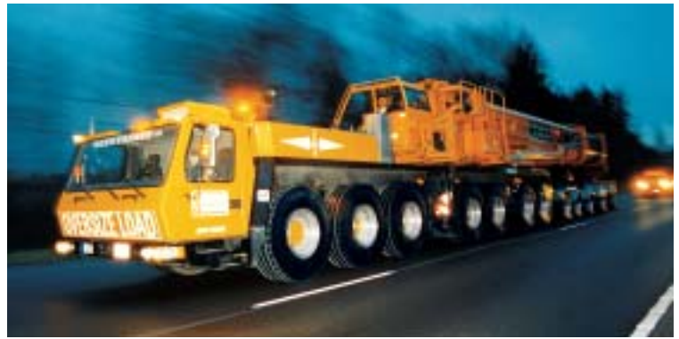
With the acquisition of Grove, Manitowoc not only filled a key void in its product offering, but gained additional global manufacturing and distribution capabilities. Shown here is the GMK 7550, a 550-ton capacity all-terrain crane, which is the largest mobile crane Grove has ever produced.
