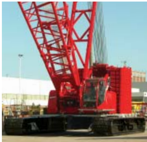
Manitowoc's Model 15000 was launched in March 2004. This 275-ton capacity crawler crane was designed in the Czech Republic and built in Germany for the European market. It expands the technology used in Manitowoc's best-selling Model 999, including its ease of transport and fast assembly capabilities.
