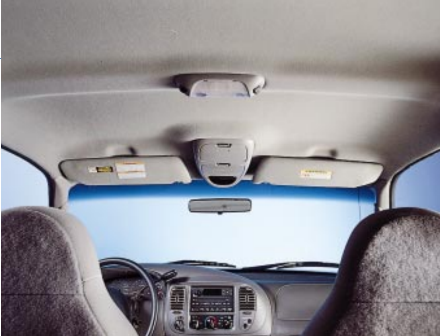
Multilayered interior headliners improve the sound insulating qualities of car roofs.
