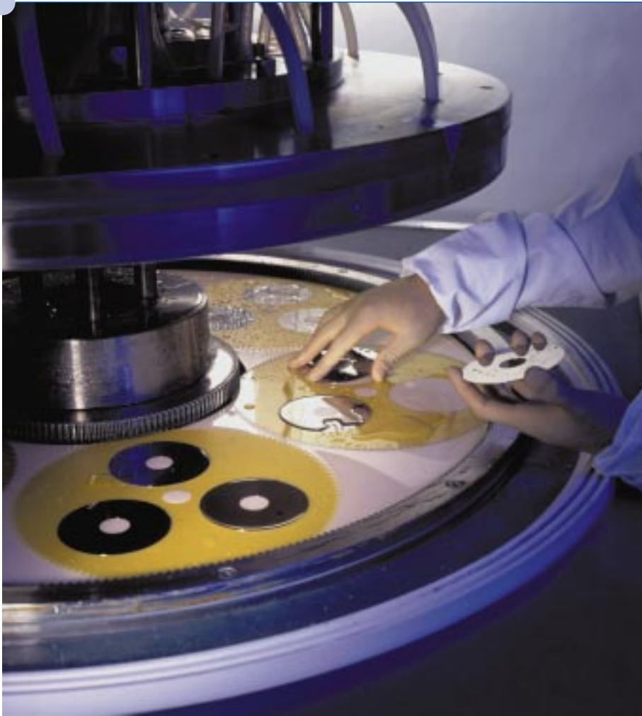
Rodel's expertise in pads and slurries makes them a leader in chemical mechanical planarization technology used to make integrated circuits.
