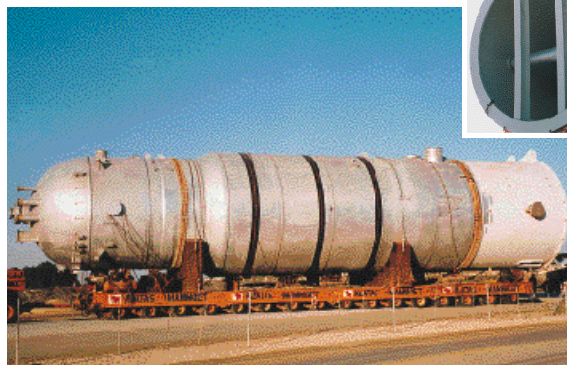
NGL stripping column - Abqaiq refinery - Saudi Arabia
