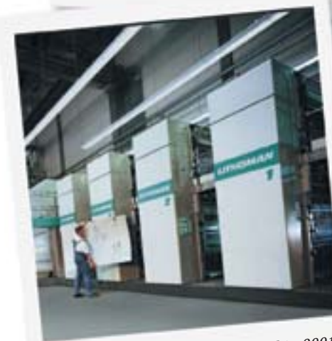
Today... The MAN Roland, installed in 2001, can produce 13 billion FSI pages a year.
