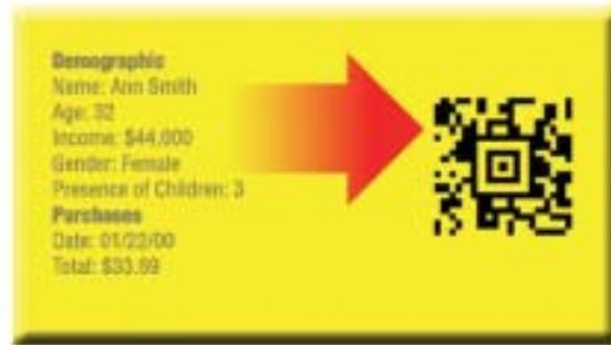
One class of CRM programs is enabled, in part, by the Aztec Code, a two-dimensional bar code that captures unique customer data.
