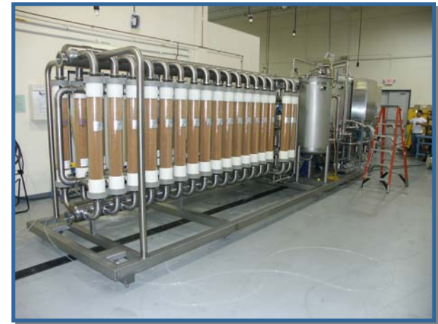
Pall Oenoflow™ systems clarify wine after fermentation to yield a clear and stable wine
