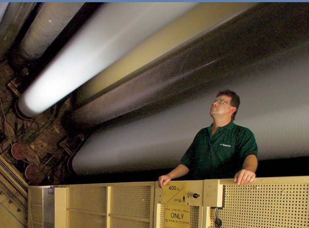
No. 3 Paper Machine calendering section at Catawba – Harold Ward, Fourth Hand, No. 3 Paper Machine.
