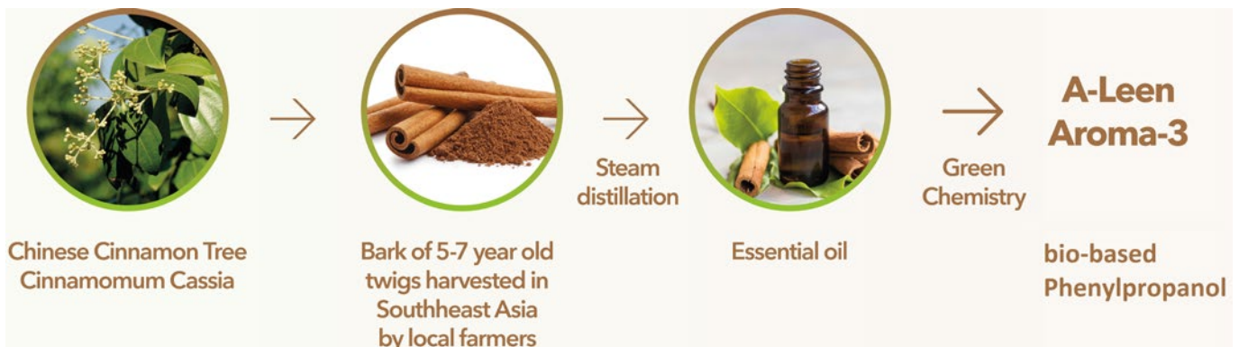
figure 2: Production of phenylpropanol from cassia bark oil.
