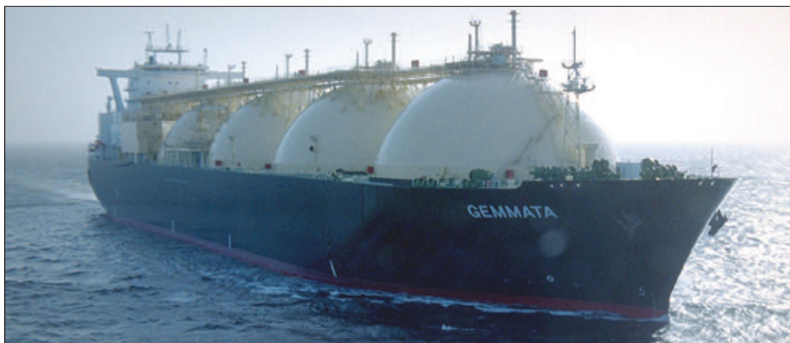
Shell's newest LNG tanker is the Gemmata , which has a capacity of 135,000 cubic metres and was delivered in January 2004. The Gemmata uses Moss Rosenberg nickel steel tanks and was built by Mitsubishi Heavy Industries in Nagasaki, Japan.
