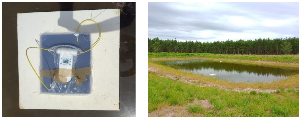
Figure 4: Installation for flux measurements (aquatic chamber) Source: Alexandre Fouache, 2022
