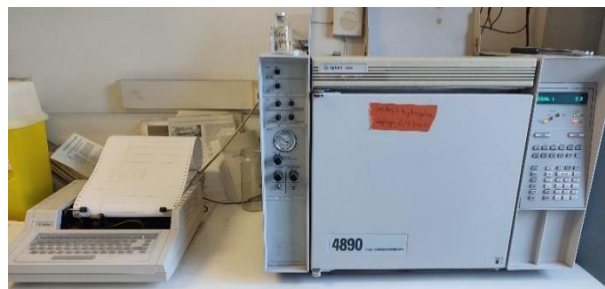
Figure 6: Gas chromatograph installation Source: Alexandre Fouache, 2022
