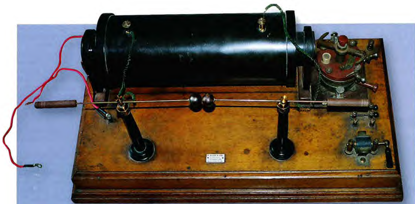
A low-power spark gap transmitter from the early 1900s. The technology was crude by today's standards but signals from high-power transmitters could be received hundreds (and sometimes thousands) of kilometres away.
