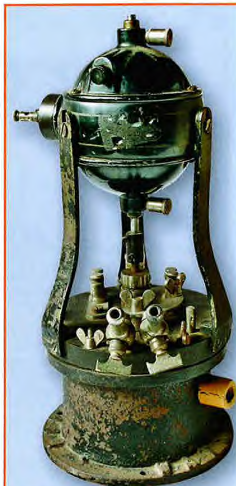
This rather strange looking device is all that remains of an old quenched spark gap transmitter.
