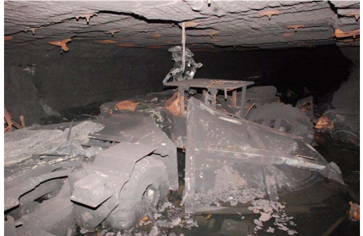
A scoop located on the Headgate 22 section after the April 5 explosion
