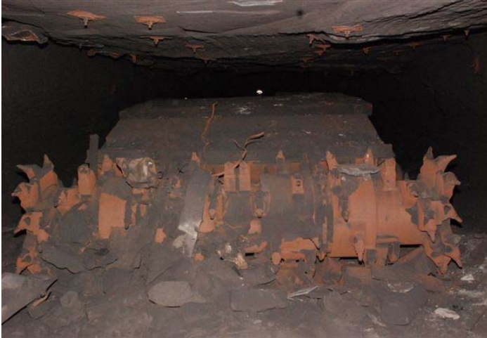
A continuous miner inside the Upper Big Branch mine after the April 5 explosion
