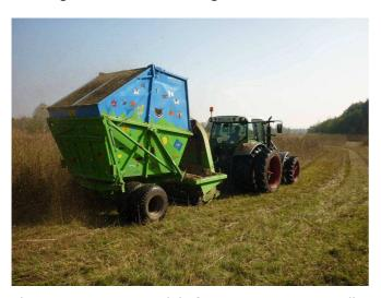
Furthermore a special mowing mobile was bought in the course of the LIFE project. That mobile can complete mowing and loading in one operational step and its soil pressure is very low. With the help of that mowing mobile even the maintenance of very wet meadows is ensured in the long run. Farmers can rent that mobile for a reasonable price.
