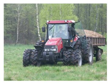
Woodchip removal using tractor with double tires for working on wet areas  $\ensuremath{\mathbb{C}}$  CMOK archive
