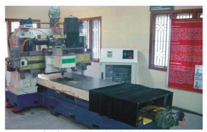
Fig-42. Computer numerical controlled eco-friendly welding machine
