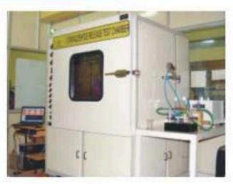
Fig-59. Formaldehyde Emission Test Chamber in IPITRI
