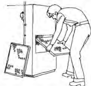
Check furnace filter
