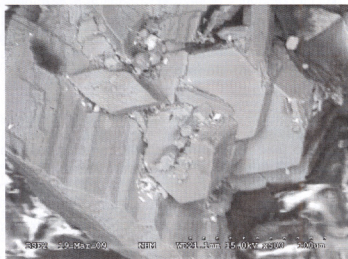
Fig. 7. SEM-photo. Hexagonal oftedalite crystals (photo Harald Folvik).
