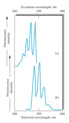
**FIGURE 15-9** Fluorescence spectra for 1 ppm anthracene in alcohol: (a) excitation spectrum and (b) emission spectrum.
