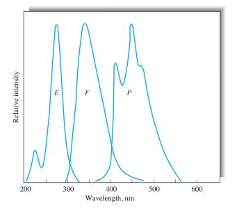
**FIGURE 15-5** Spectra for tryptophan: *E*, excitation; *F*, fluorescence; *P*, phosphorescence. (Adapted from G. G. Guilbault, *Practical Fluorescence*, New York: Marcel Dekker, 1973, p. 164. Courtesy of Marcel Dekker, Inc.)
