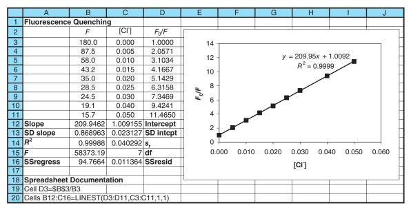
FIGURE 15-4 Spreadsheet and plot to determine quenching constant for chloride ion quenching of quinine.
