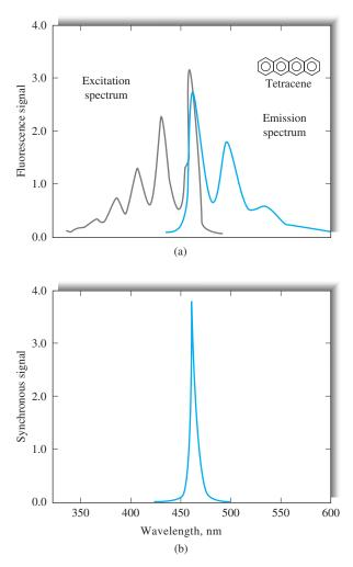
FIGURE 15-7 Synchronous fluorescence spectra. In (a), the excitation and emission spectra of tetracene are shown. In (b), the synchronous spectrum is shown for a fixed-wavelength difference of 3 nm. (From T. Vo-Dinh, *Anal. Chem.*, **1978**, *50*, 396, **DOI**: 10.1021/ac50025a010. Figure 1, p. 397. Copyright 1978 American Chemical Society.)
