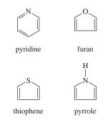
do not exhibit fluorescence. On the other hand, fused-ring structures ordinarily do fluoresce. With nitrogen heterocyclics, the lowest-energy electronic transition is believed to involve an  $n \rightarrow \pi^*$  system that rapidly converts to the triplet state and prevents fluorescence. Fusion of benzene rings to a heterocyclic nucleus, however, results in an increase in the molar absorptivity
