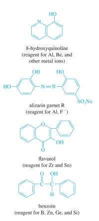
**FIGURE 15-15** Some fluorometric chelating agents for metal cations. Alizarin garnet R can detect  $Al^{3+}$  at levels as low as 0.007 µg/mL. Detection of F<sup>-</sup> with alizarin garnet R is based on fluorescence quenching of the  $Al^{3+}$  complex. Flavanol can detect Sn<sup>4+</sup> at the 0.1-µg/mL level.
