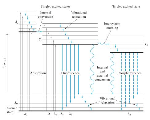
FIGURE 15-2 Partial energy-level diagram for a photoluminescent system, often called a Jablonski diagram.
