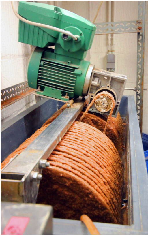
Figure 11.3 Lab-Scale OLAND-rotating biological contactor at the Laboratory of Microbial Ecology and Technology (Ghent University), started up in 2000 (Pynaert et al. , 2002). Picture from 2014.
