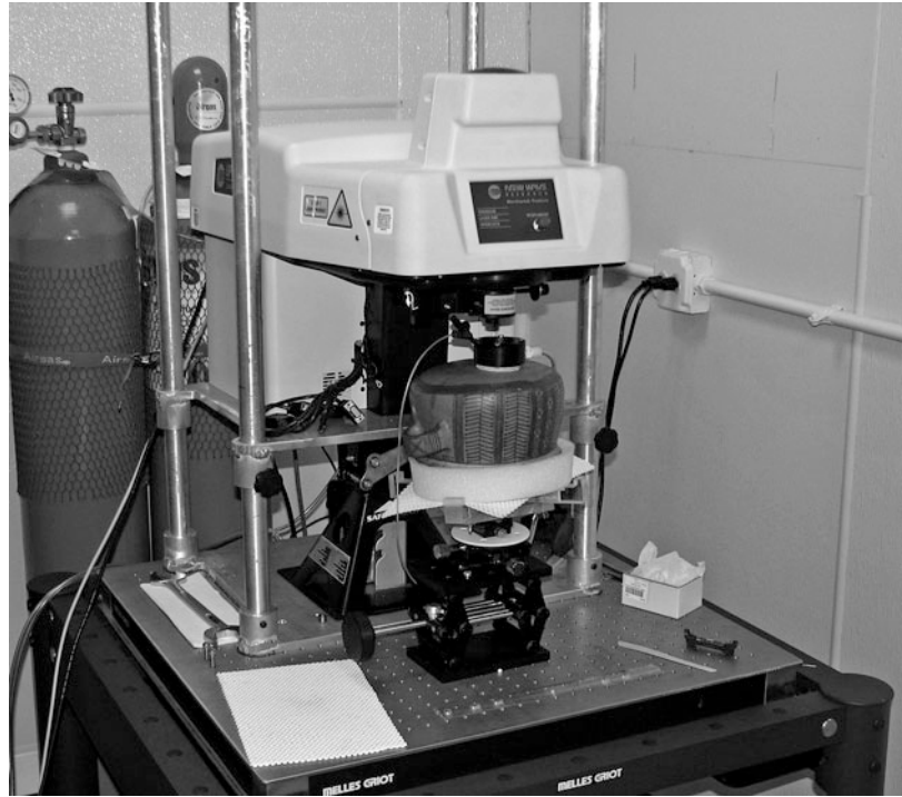
Fig. 3.1 The Field Museum's open-cell laser, a New Wave Micro 266 laser modified to seal to large objects. An Inka style ceramic vessel (FM2765) is positioned for analysis
