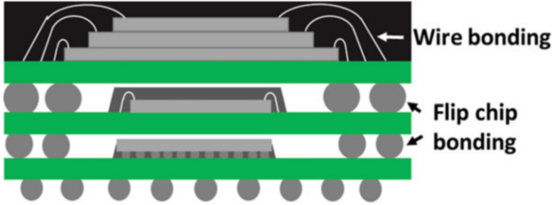
Fig. 1.10 Schematic illustration of package-to-package 3D integration (adapted from Ref. [3])
