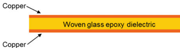
Fig. 11.7 Schematic cross section: organic substrate core material
