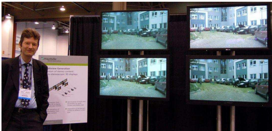
Ralf Tanger of the HHI (Heinrich Hertz Institute) branch http://www.hhi.fraunhofer.de of the world famous German R&D institute Fraunhofer (both with long histories of 3D projects) showing their new autostereoscopic server software playing from one file on 42 inch panels from four different auto panel makers--Tridelity www.tridelity.de (5 view barrier), Alioscopy www.alioscopyusa.com (8 view lenticular), NewSight www.newsight.com (8 view barrier) and Philips (terminated this product line a year ago) (9 view lenticular). Fraunhofer has been researching 3D for at least a decade and the HHI long before that. They also showed multiview synthesis from two views (e.g., from a stereo
