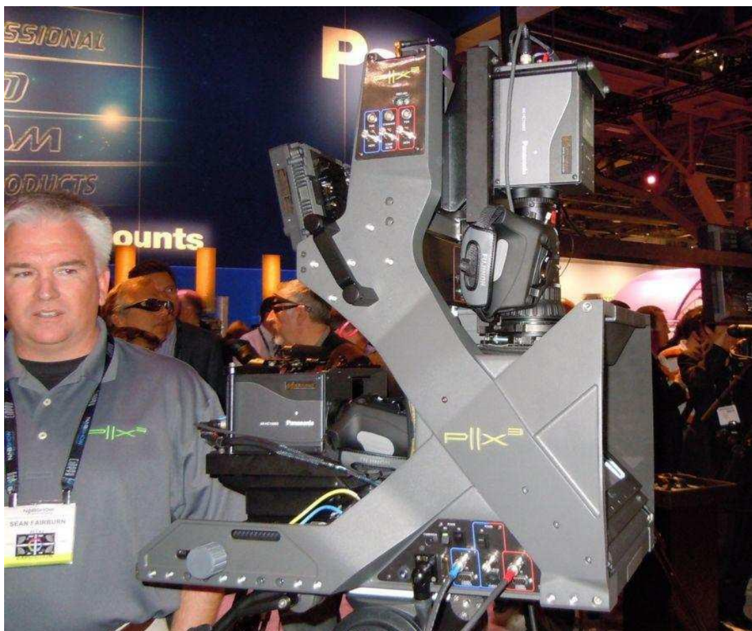
Sean Fairburn with the PX3 Renegade Solution Camera Rig of PLLX3 (Parallax 3) in the Panasonic booth http://www.pllx3.com/px3.htm . It has a wireless remote, for cam and lens controls, a DVI 3D out in 3 formats, and 2 configurable 3D outs including subtractive overlay (for alignment). Based in California, they (principally Bradley Nelson who also helped design the 3D laser projector in the Hdlogix booth) also made the 30 x 90ft 3D LED video wall for Michael Jackson's ill fated This is It
