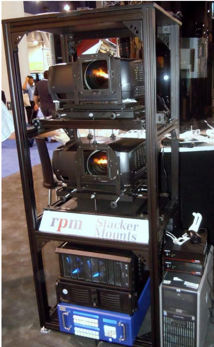
Equipment distributor RPM showed dual CP projection with their Stacker Mounts and images from a PC via two eyeVis openWarp processors.
