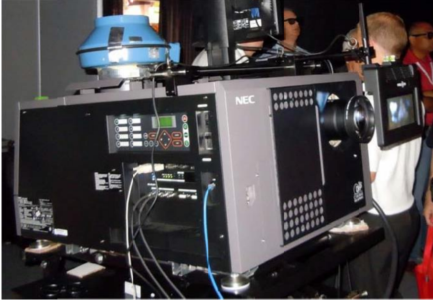
The newest NEC Staurus 3 Chip DLP Cinema Projector with a RealD XL CP switch—currently the world’s brightest 3 chip.
