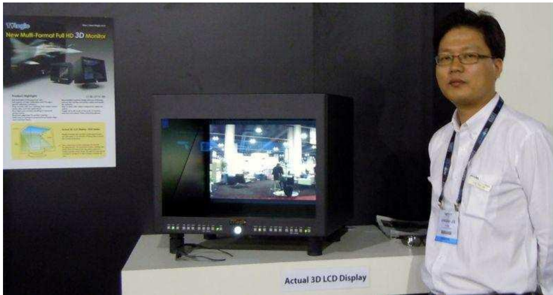
Mr Lee of TV Logic with their new full HD polarized monitor consisting of dual LCD's with semisilvered mirror.
