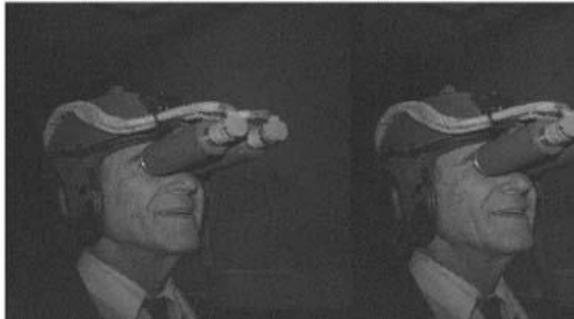
High resolution field sequential color prototype using Tektronix NuColor LCD elements shown by Tektronix at Siggraph 1992.
