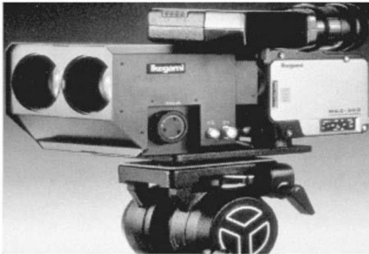
Ikegami's original stereo zoom camera in 1990 cost $90,000 & has been improved by them & several of it's users.
