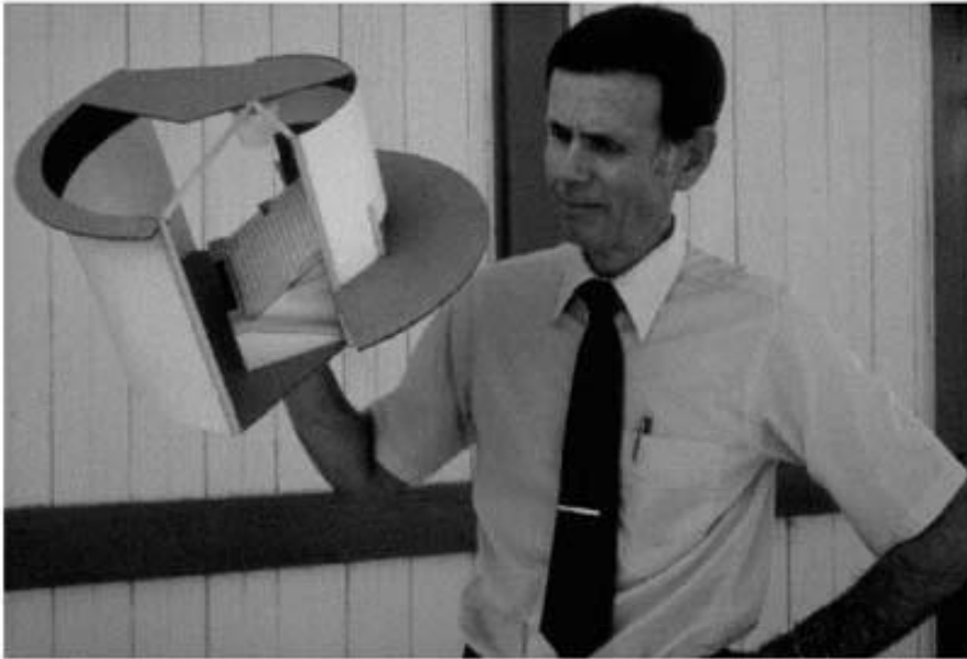
Inventor Robert Collender in 1978 with a model of his StereoptiPLEXer autostereoscopic 3D theater. In his small working model, the images came from a single 16mm filmstrip and were scanned onto the vertically brushed stainless steel screen with a rotating polygon but his later patents described totally electronic systems.
