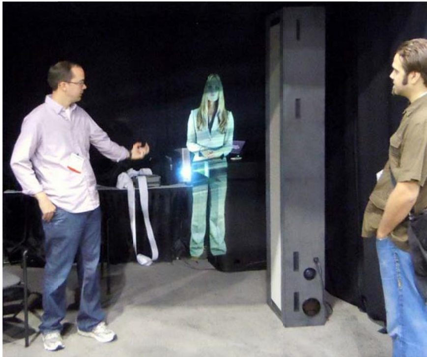
The Fogscreen projects on a very fine water mist and has been used in 3D with
