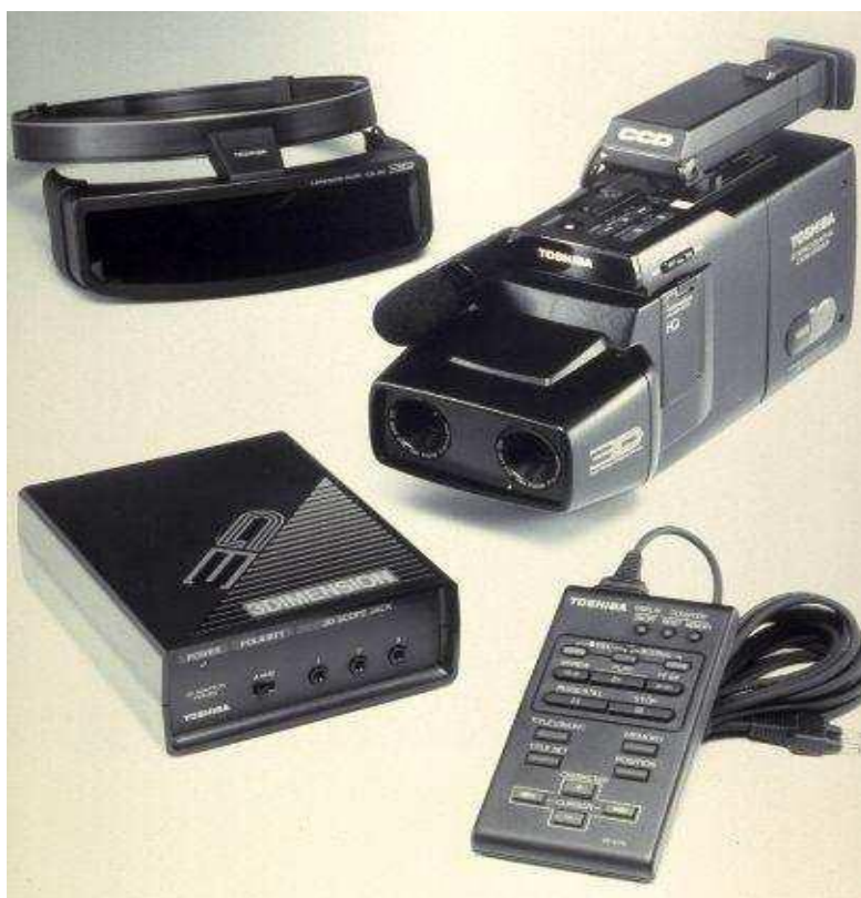
Toshiba 3D Camcorder system of which 500 were made in 1988. I still use them occasionally with recording on digital via its composite video out. I converge and focus the lenses as close as 8 inches using single 72mm diameter closeup diopters on
