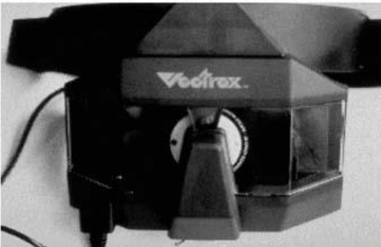
Three pioneering stereo products.(TOP) Vision Research Graphics original kit for IBM PC(1990). (MIDDLE) 1990 version of 3DTV Corp StereoDemultiplexer for converting field sequential 3D video into right & left channels. (BOTTOM) 1984 Vectrex visor with spinning color wheel converted 2D monochrome vector graphics into field sequential color stereo.
