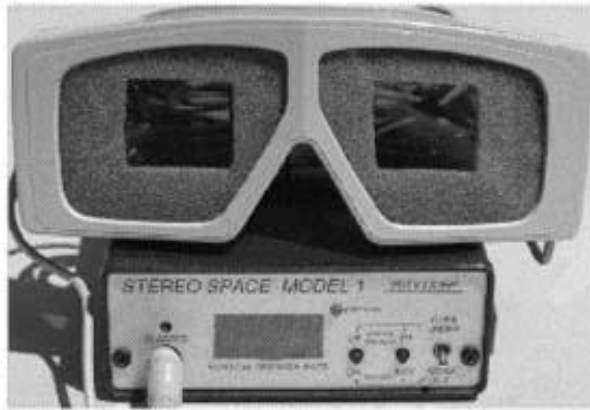
LCD shutter glasses & 3DTV Corp's StereoSpace Model 1 sync pulse inserter with digital frequency counter for use with above/below stereo format on PC's with programs like Worldtool Kit, VREAM, Division, SuperScape etc. Recent improvements in hardware make this the leading contender for stereo imaging on PC's since it's compatible with every operating system & nearly all hardware.
