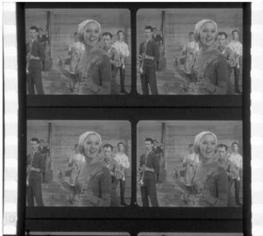
The side by side square format used by the Russian Stereo 70 camera and projection system from the 1970's to the present. About real size.
