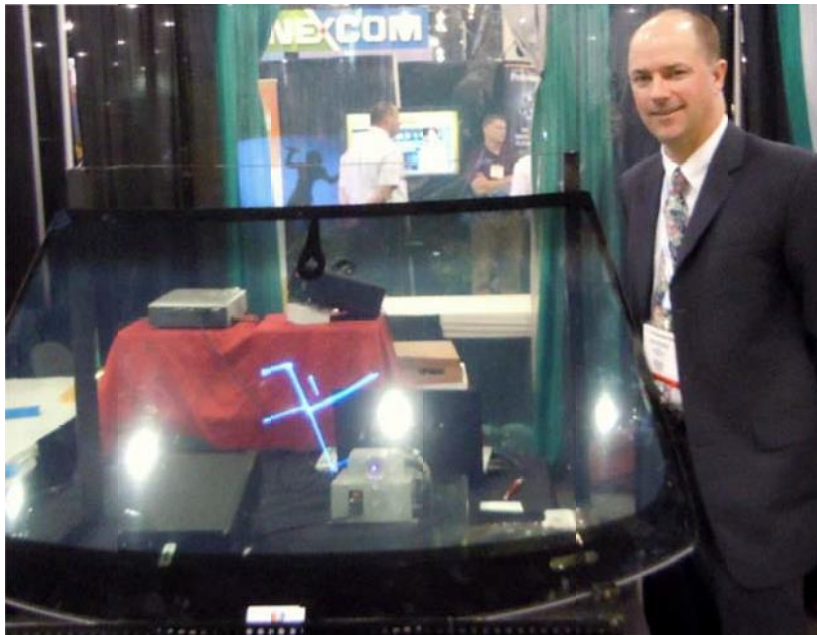
Doug Bragdon of Superimaging Inc- Fremont, Calif. USA www.superimaging.com demonstrates their UV laser addressed two color displays made by applying a special fluorescent nanoparticle film to any clear medium. The small sized HUD TransPlay projector is shown here in the Smart
