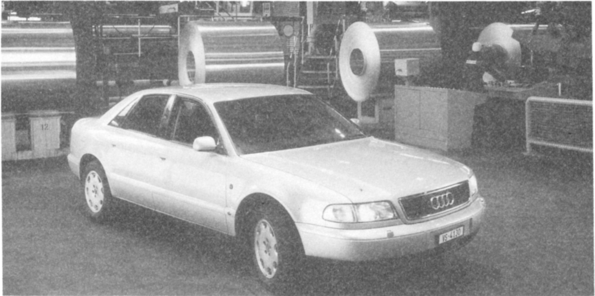
Figure 18.3 The Audi A8 Luxury Saloon. All-aluminium spaceframe construction. (Courtesy of the Aluminium Extruders Association.)
