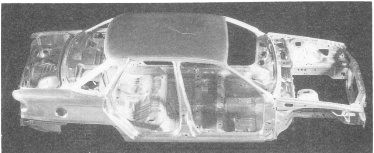
Figure 18.2 The unitary construction of the Ford aluminium intensive vehicle. (Courtesy of the Aluminium Extruders Association.)
