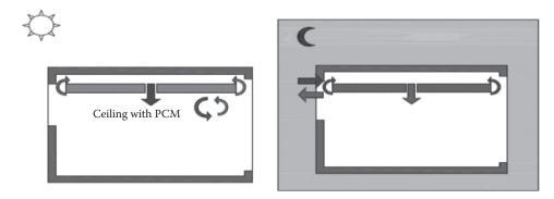
FIGURE 7.10 General concept of cooling with PCM integrated into ceiling.
