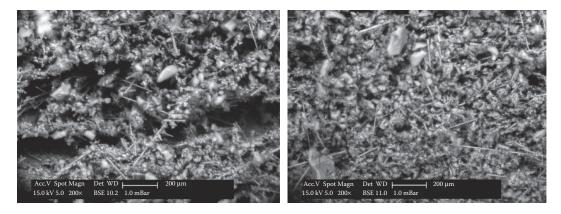
FIGURE 8.3 SEM images of an aerogel blanket.
