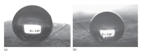
FIGURE 8.7 Water droplet on NGF aerogel blanket (a) and NGF wool (b).
