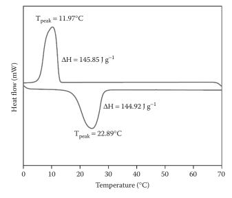
**FIGURE 7.16** DSC curve of the eutectic PCM.
