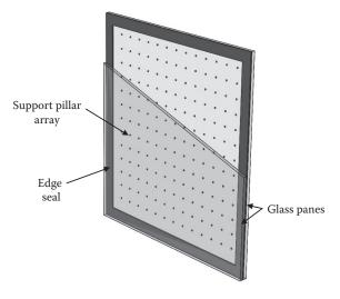
**FIGURE 4.2** Schematic diagram of a vacuum glazing.
