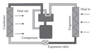
FIGURE 12.5 Basic heat pump configuration.
