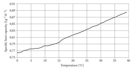
**FIGURE 8.10** Specific heat of the NGF aerogel blanket.
