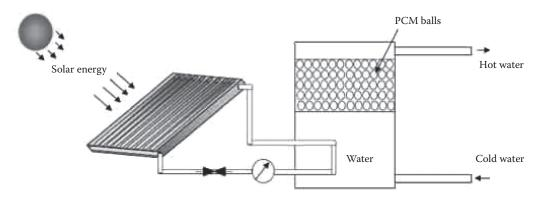
**FIGURE 7.3** Domestic hot water system with PCM thermal energy storage.
