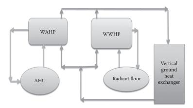
**FIGURE 2.6** Overall HVAC system diagram for ZØE.
