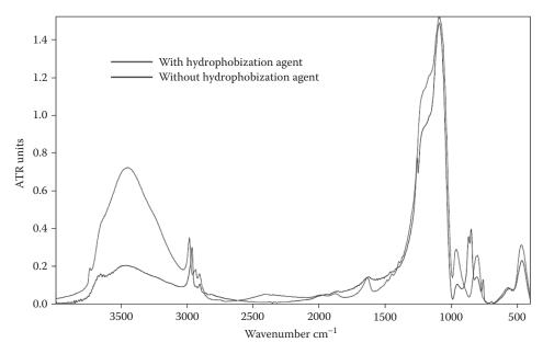
**FIGURE 8.5** FTIR spectra of silica aerogel phase.
