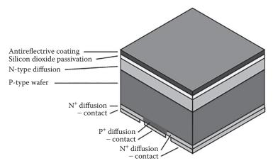
**FIGURE 6.3** Single-crystalline silicon solar cell.
