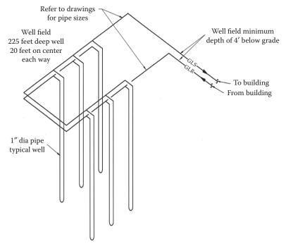
**FIGURE 2.4** Vertical ground loop heat exchanger.
