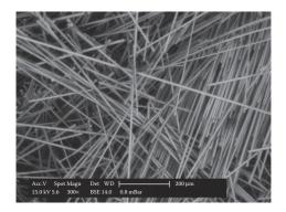
**FIGURE 8.2** SEM image of a needle glass fibers wool.
