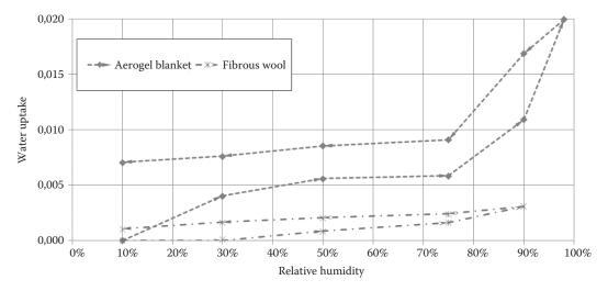
**FIGURE 8.6** Sorption and desorption curve of the aerogel blanket.
