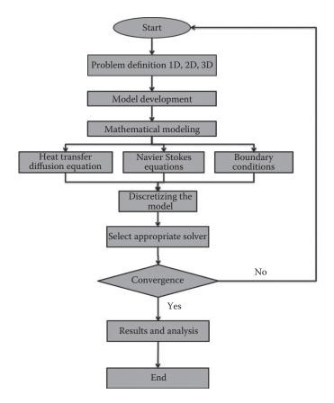
**FIGURE 11.5** Flow diagram for CFD analysis.
