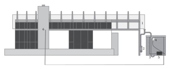
The schematic diagram of rainwater harvesting system of the ZØE lab: 1—roof funnel; 2—mesh filter; 3—pressure transducer; 4—main controller; 5—sediment filter; 6—carbon filters.
