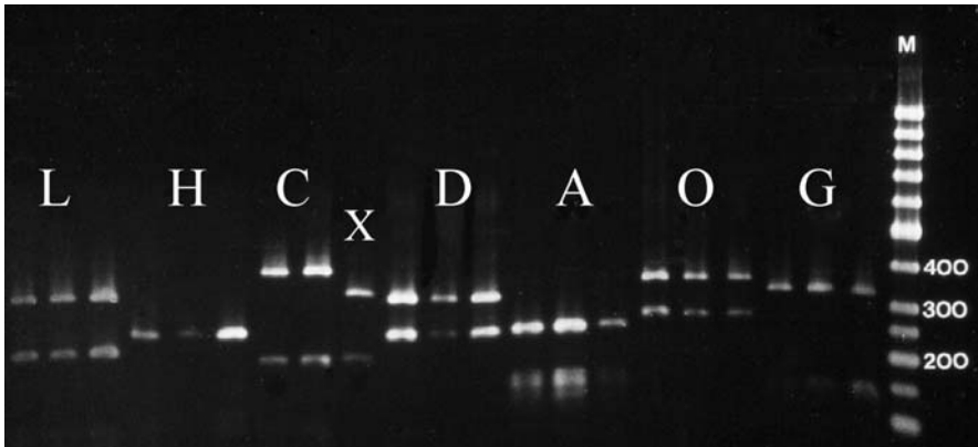
Fig. 2.21. Species-specific ITS-RFLP pattern of isolates of Serpula lacrymans (L), S. himantioides (H), Coniophora puteana (C), Donkioporia expansa (D), Antrodia vaillantii (A), Oligoporus placenta (O), and Gloeophyllum sepiarium (G) generated by TaqI . M marker (50–1,000 bp). The culture X had been assumed to be C. puteana and was later identified by sequencing as C. olivacea
