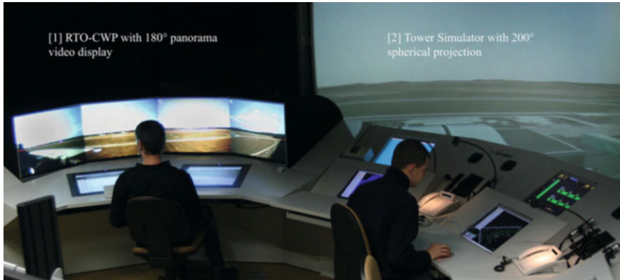
Fig. 1 The experimental workplace for remote tower operations (RTO-CWP) [1] integrated within the infrastructure of the conventional tower simulator [2] (IEEE copyright)
