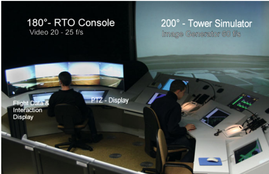
Fig. 12 RTC simulator environment used for remote tower experiments [reprinted from Fürstenau et al. (2011), IFAC, with permission]. Photo depicts the previous 200° vision system of the DLR tower simulator (ATS), extended by the 180° RTO backprojection console ( left ). The latter could alternatively display RTO simulations or the live panorama
