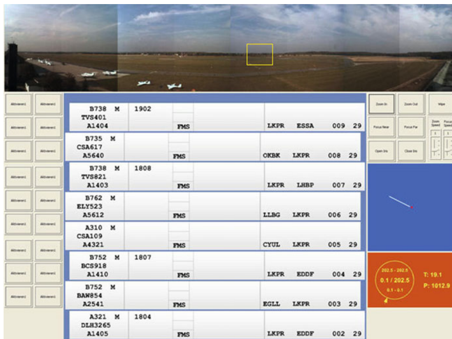
Fig. 6 Initial design of pen touch-input interaction display [reprinted from Schmidt et al. (2009), IEEE, with permission]. Minipanorama on top as option for PTZ positioning via touch (actual position visualized by yellow square). Center, electronic flight strips; right, from top, PTZ control buttons, virtual joystick as another option for PTZ positioning, weather data with wind direction (from weather sensors); left, optional buttons, e.g., for preset PTZ position
