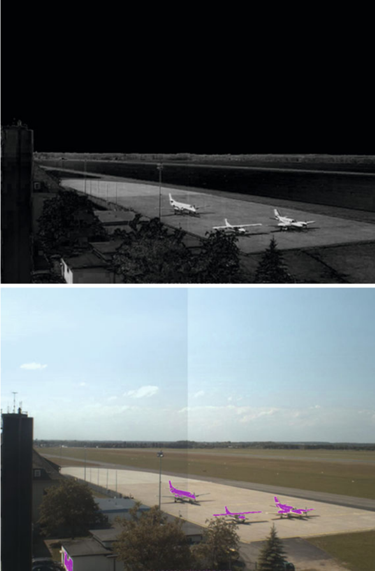
Fig. 9 Bright color feature characterizing aircraft (upper b/w image, Braunschweig panorama camera 3). Lower image: colored overlay results depict detected objects including one false positive on the left side, indicating the necessity of additional features for discrimination, e.g., area restrictions
