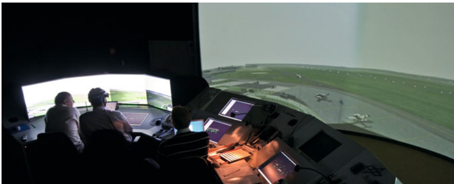
Fig. 5 RAiCe1 setup: remote tower console (left) and 200° projection system (right)
