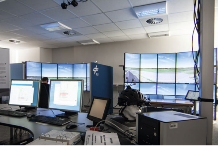
Fig. 11 Multi-remote tower setup ( left , single working position; right , multi-remote working position)
