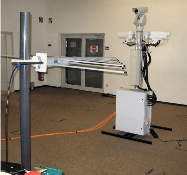
Fig. 12 Experimental setup for measuring electromagnetic emission
