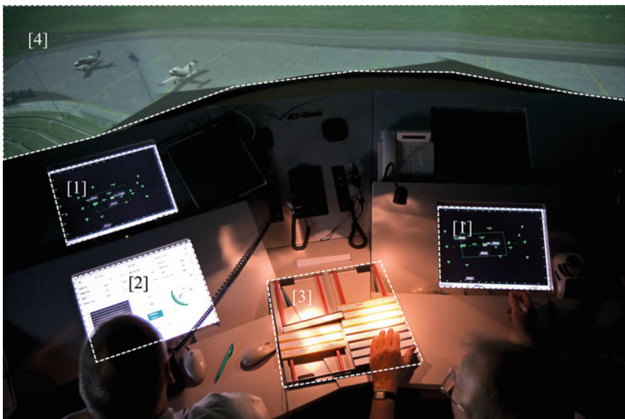
Fig. 2 Design of working positions in the tower simulator encompasses [1] two radar displays, [2] weather display, [3] flight strips, and [4] far view (200° life-size projection). The executive is positioned to the left and the coordinator to the right of the flight strips
