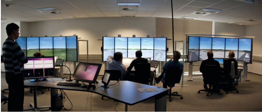
Fig. 10 Remote tower center (RTC) design for controlling three airports from afar. Foreground, ground coordinator; back, three airport CWPs for executive controllers
