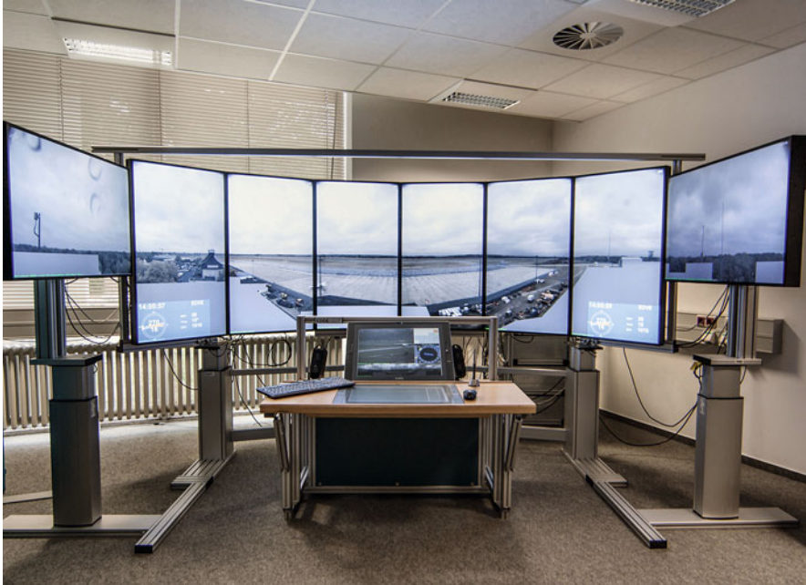
Fig. 3 Prototype RTO-Videopanorama with basic controller console in the DLR Tower-Lab (2013) reproducing the out-of-windows view at Braunschweig airport. 360° horizontal FOV with 6 vertical displays for the 228° view towards the runway in northern direction. Two horizontal displays covering the southern 136° viewing sector with the same resolution
