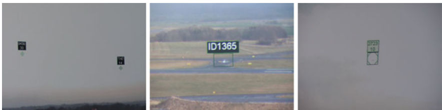
Fig. 5 Left : Aircraft tracked only by the terminal approach radar (labels with call sign or SSR code and altitude in hundreds of feet); Middle : aircraft tracked by the video camera only (label with track number); Right : aircraft tracked by both radar and video
