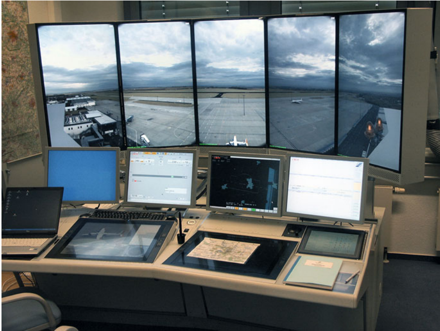
Fig. 4 Implementation of the R-CWP at Erfurt tower control room without direct airport view. Three levels of information with the videopanorama in the back, the row of four flight information displays, operator console with two large touch-input displays, and a small one at the right side for radio communication are clearly structured (for details see text)
