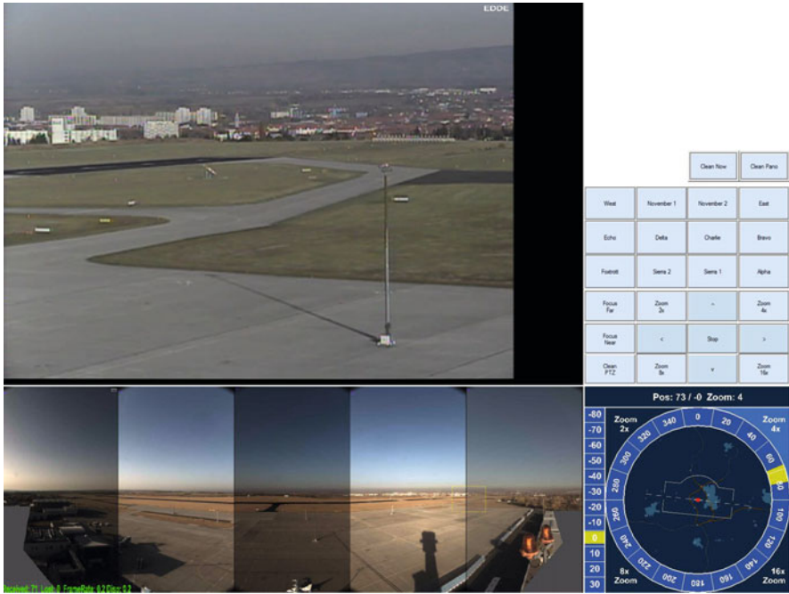
Fig. 6 Pan-tilt-zoom camera control pen-touch input display with viewing direction indicator (virtual joystick, bottom right) including zoom factor selection ( Z=2, 4, 8, 16 ) and mini-panorama. For details see text
