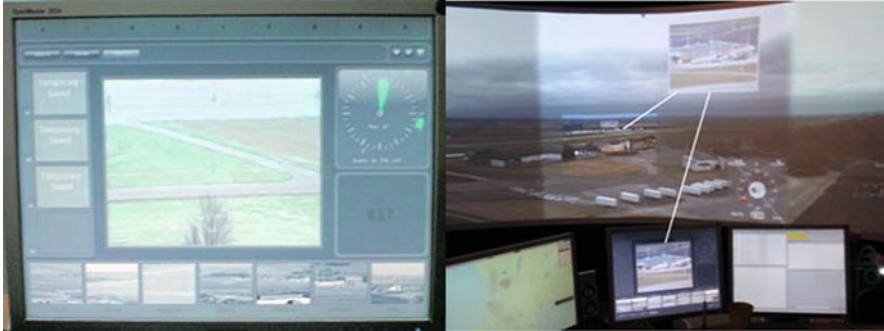
Fig. 6 PTZ camera human machine interface ( left ) and picture-in-picture ( right )
