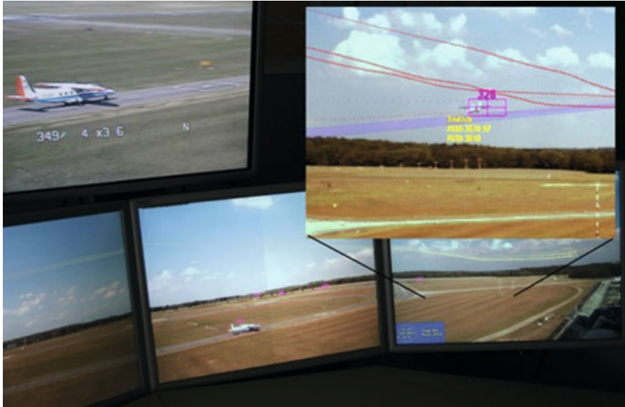
Fig. 7 Part of the initial version of the panorama display with PTZ display on top. Inset: screenshot of camera #4 (= east) display showing augmentation during landing [reprinted from Schmidt et al. (2009), IEEE, with permission]. Superimposed glide path ( violet , added for replay), GPS trajectories ( red ), live multilateration position ( yellow , from transponder), and automatic movement detection ( red square with object number)
