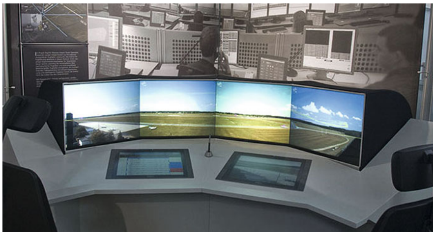
Fig. 5 Experimental RTO videopanorama (180°) backprojection system. It was installed in the RTO simulator environment (see Sect. 5) and could display simulated as well as live traffic (the latter shown in the photo). PTZ display is integrated in the console (right side) beside the interaction and camera control display on the left (Sect. 3.3). Reprinted from Schmidt et al. (2009), IEEE, with permission
