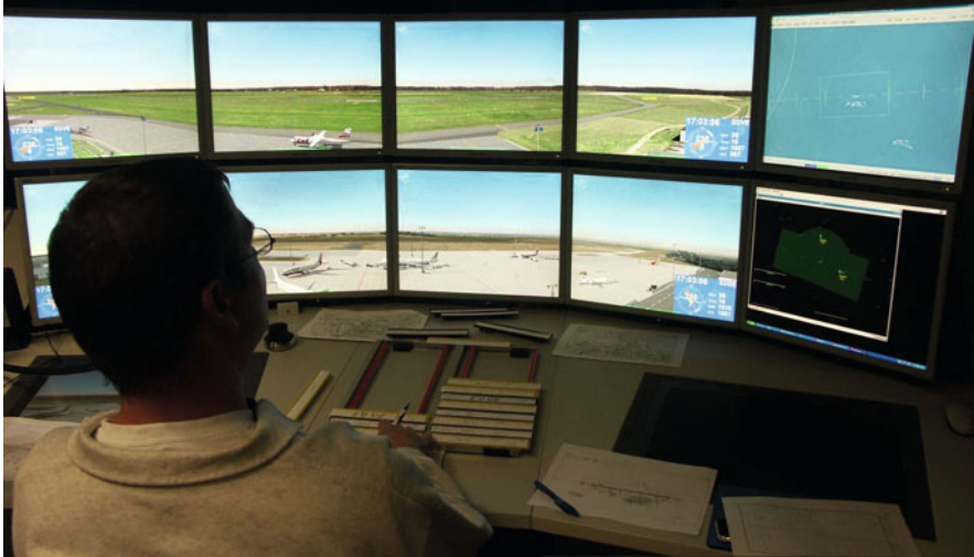
Fig. 13 RTC simulator setup for human-in-the-loop simulation with simultaneous surveillance of two remote airports using two augmented vision videopanorama systems
