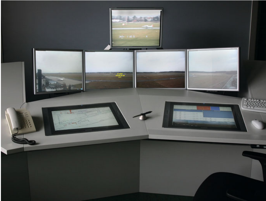
Fig. 4 Early version of 180° videopanorama (1600 × 1200 pixel) with pan-tilt-zoom camera display on top, demonstrating augmented vision function: superimposed transponder label tracking the landing aircraft using automatic movement detection (see Sect. 3.4, Fig. 7). Two pen touch-input displays integrated in the console display additional information required by the controller: the one on the right was used for electronic flight strips (flight data) and control of the camera parameters, PTZ, weather information, and tracking. Initially published in Fürstenau et al. (2007)
