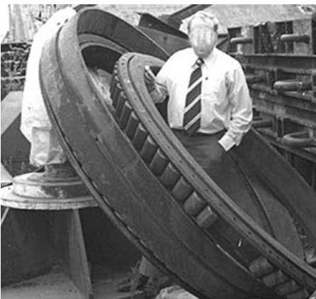
Figure 2.10 Broken main bearing of the MRTA tunnelling machine
