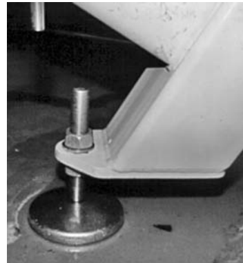
Figure 2.24 Photograph of a typical leg support pad
