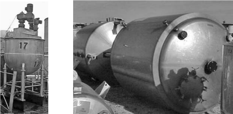
Figure 4.23 An early design of industrial pressure cooker and a current form of industrial pressure cooker being used as a horizontal autoclave
