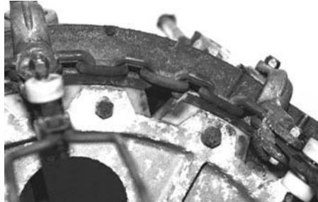
Figure 1.9 Chickweigh line corner pulley showing shackles fitting into slots on wheel
