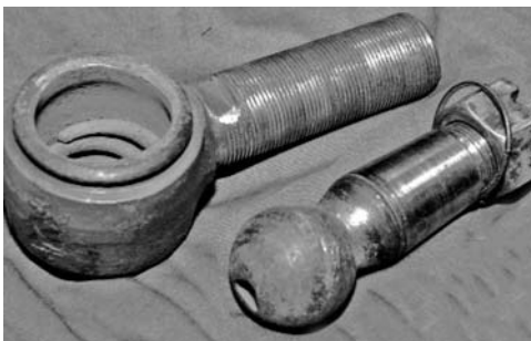
Figure 2.71 The failed ball joint on the steering link. The socket had been cleaned out for this photo
