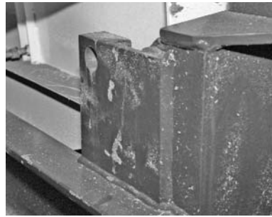
Figure 3.21 Close-up view showing some of the weld runs on the machine frame
