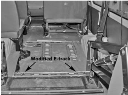
Figure 3.36 Modified E-track installed in a transport vehicle
