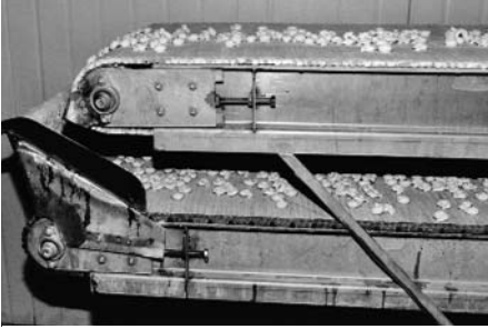
Figure 3.24 Transfer end of conveyor inside the freezing tunnel
