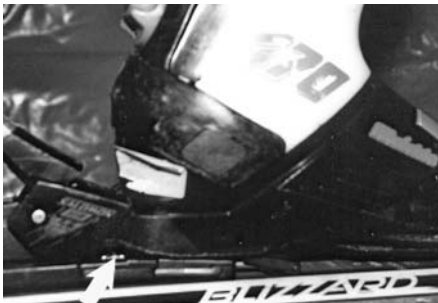
Figure 4.21 The right ski boot under forward release moment test
