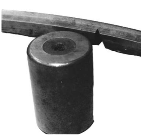
Figure 2.12 Bearing roller and part of the failed bearing cup. The notch was used for establishing material properties
