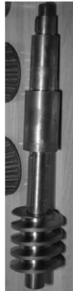
Figure 2.5 Typical motor shaft and worm screw
