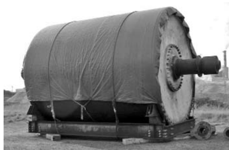
Figure 2.76 The discarded Yankee dryer stored on a field float at Marigold
