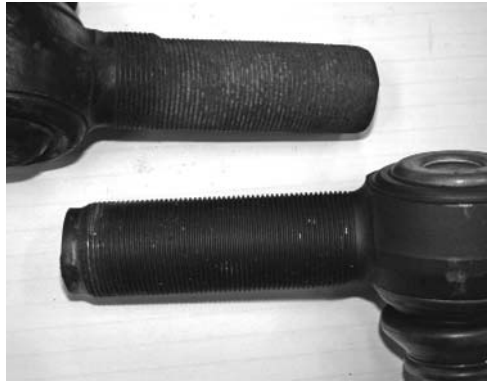
Figure 2.61 Worn knuckle (top) and new knuckle (bottom)
