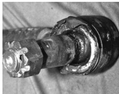
Figure 2.72 The ball joint at the other end of the steering link. Note the damaged grease boot
