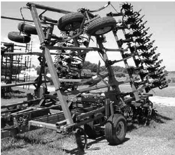
Figure 3.1 Cultivator folded for transport
