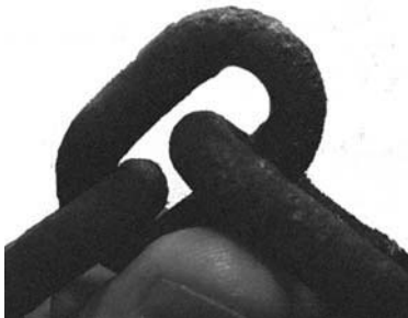
Figure 1.12 Close-up of chain showing substantial wear at the end of the link
