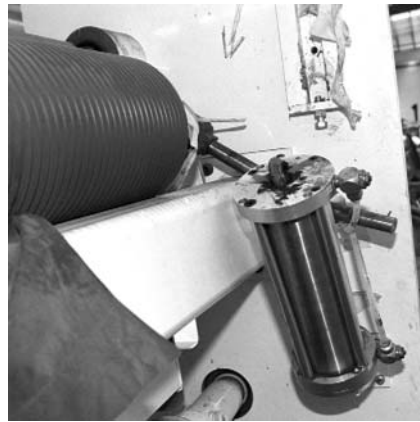
Figure 2.43 View showing roller dislodged from its bearing and damaged air cylinder
