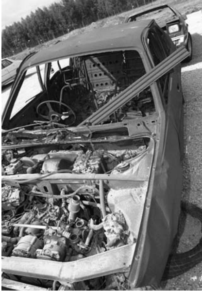
Figure 6.30 View of the burnt-out engine compartment
