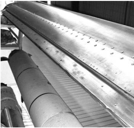
Figure 2.42 View along air delivery nozzle, with airknife blades removed
