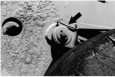
Figure 4.28 Close up view of the lift arm pivot lubricating hose
