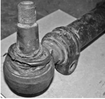
Figure 2.58 Original design of track rod (worn sample from Fillary)
