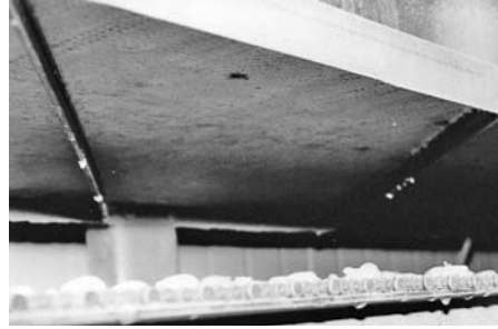
Figure 3.25 View underneath the conveyor belt showing hoar frost wipers
