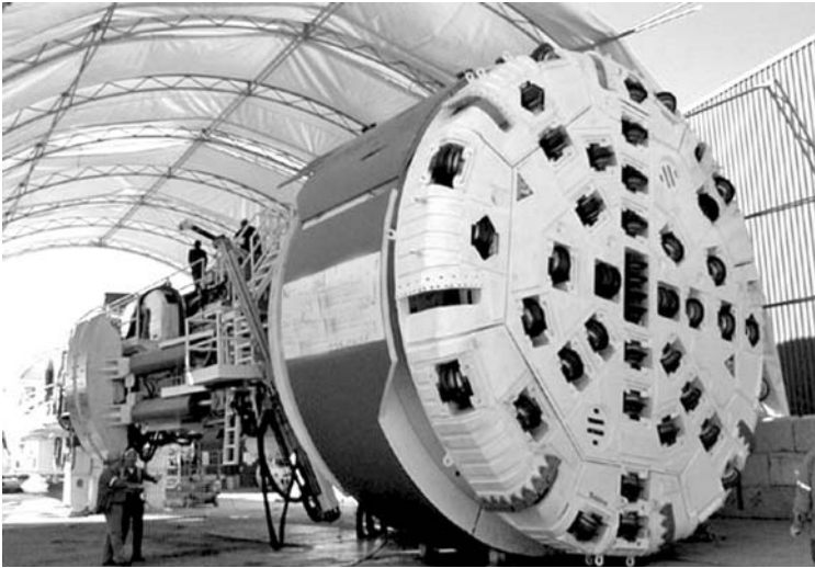
Figure 2.6 Full-face tunnelling machine just before entering tunnel portal
