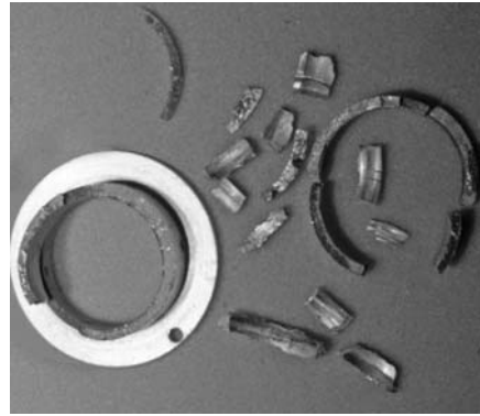
Figure 2.52 Components of bearing shell recovered from seized compressor
