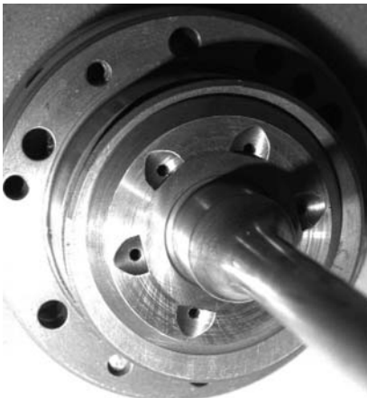
Figure 2.53 Nominally worn thrust face of high-speed shaft replaced in overhaul
