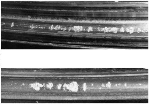
Figure 2.22 Bearing damage. The upper photo shows the damage to the inner (fixed) race. The lower photo is that of the damage to the moving (outer) race
