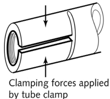
Figure 2.65 Schematic sketch of a pipe clamp designed to permit better grip on the steering knuckle thread
