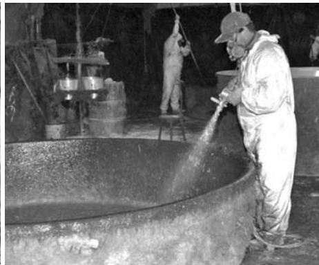
Figure 3.30 Spray-up of tank in progress
