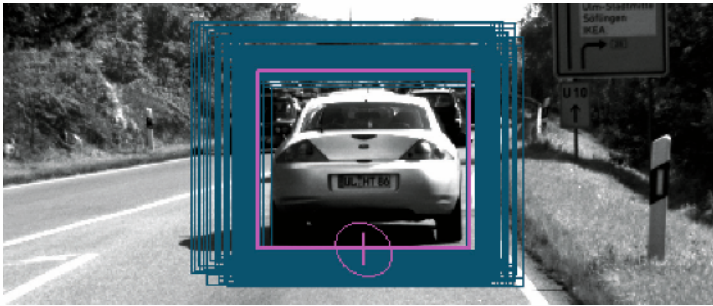
Fig. 7. The video measurement noise is determined by the empirical covariance (magenta 3\sigma ellipsoid) of the detection boxes (cyan) within a cluster.
