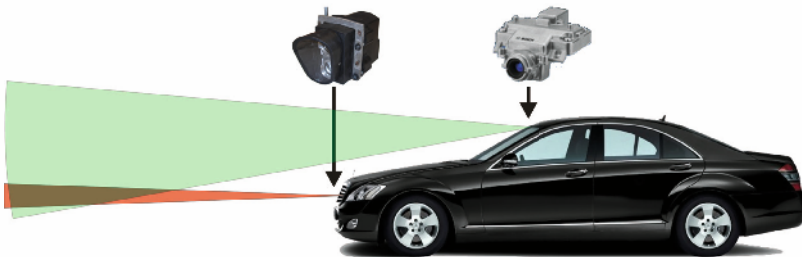
Fig. 2. Test vehicle equipped with serial nightview camera and multibeam Lidar sensor.
