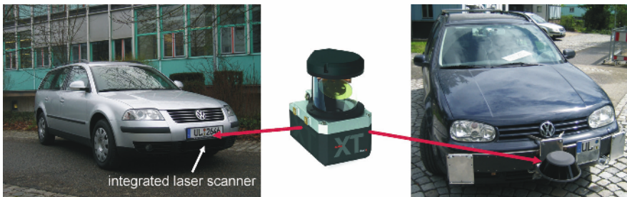
Fig. 1. The laser scanner IBEO ALASCA XT is integrated at the front bumper of the testing vehicles.
