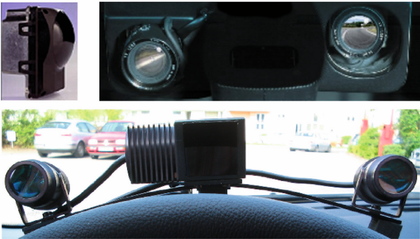
Fig. 5. Sensors: radar (top left), lane detection system (top right) and driver monitoring system
