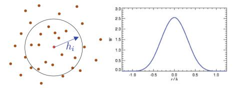
Fig. 29 Kernel interpolation with a B-spline kernel
