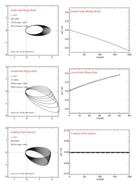
**Fig. 2** Kepler problem integrated with different integration schemes (Springel, 2005). The panels on *top* are for a 4th-order Runge Kutta scheme, the *middle* for a 2nd order Runge-Kutta, and the *bottom* for a 2nd-order leapfrog. The leapfrog does not show a secular drift of the total energy, and is hence much more suitable for long-term integration of this Hamiltonian system
