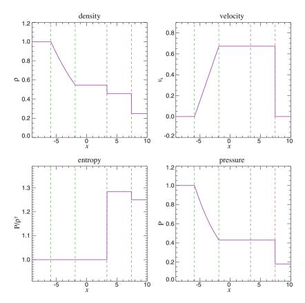
Fig. 25 Evolved state at t = 5.0 of the initial fluid state displayed in Fig. 24. The *blue dashed line* marks the position of the contact wave, the *green dashed lines* give the location of the rarefaction fan, and the *red dashed line* marks the shock
