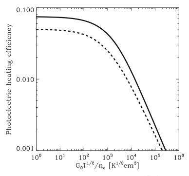
**Fig. 6** Photoelectric heating efficiency  $\epsilon$  as a function of  $\psi \equiv G_0 T^{1/2} n_e^{-1}$ . Values are plotted for gas temperatures of 6000 K (*solid line*), characteristic of the WNM, and 60 K (*dashed line*), characteristic of the CNM. The values shown here are based on the work of Bakes and Tielens (1994), as modified by Wolfire et al. (2003). In the local ISM,  $\psi \sim 2 \times 10^4$  in the WNM and ~2000 in the CNM (Wolfire et al. 2003)
