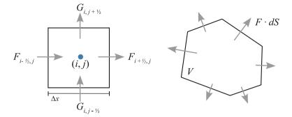
Fig. 27 Sketch of unsplit finite-volume update schemes. On the *left*, the case of a structured Cartesian grid is shown, the case on the *right* is for an unstructured grid
