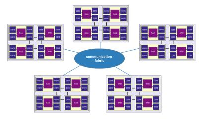
Fig. 35 In large high-performance supercomputers, one typically connects a large number of powerful compute nodes (often of NUMA type) through a very fast dedicated communication network
