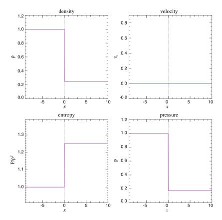
Fig. 24 Initial state of an example Riemann problem, composed of two phases in different states that are brought into contact at x = 0 at time t = 0. (Since  $v_x = 0$ , the initial conditions are actually an example of the special case of a Sod shock-tube problem)
