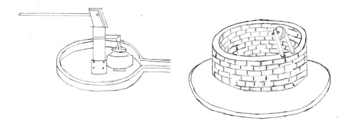
**Open Well**: Where ground water is available at low depth (less than 15 meters - and water is available all year round, open well is used.
