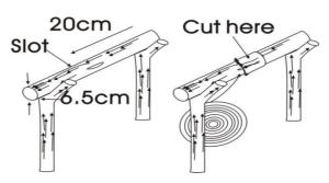
Figure 4 Pot cutting roll
